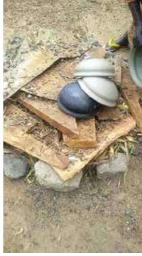
Plate 29 Fired/green wares staking Field generated Photograph.
