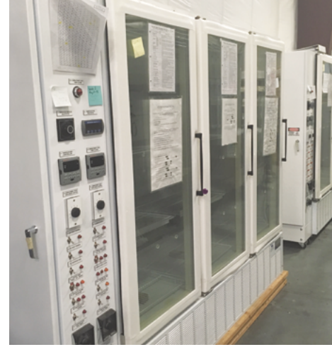
Blast freezers used to eliminate pest infestations and to freeze dry water-damaged collections.
