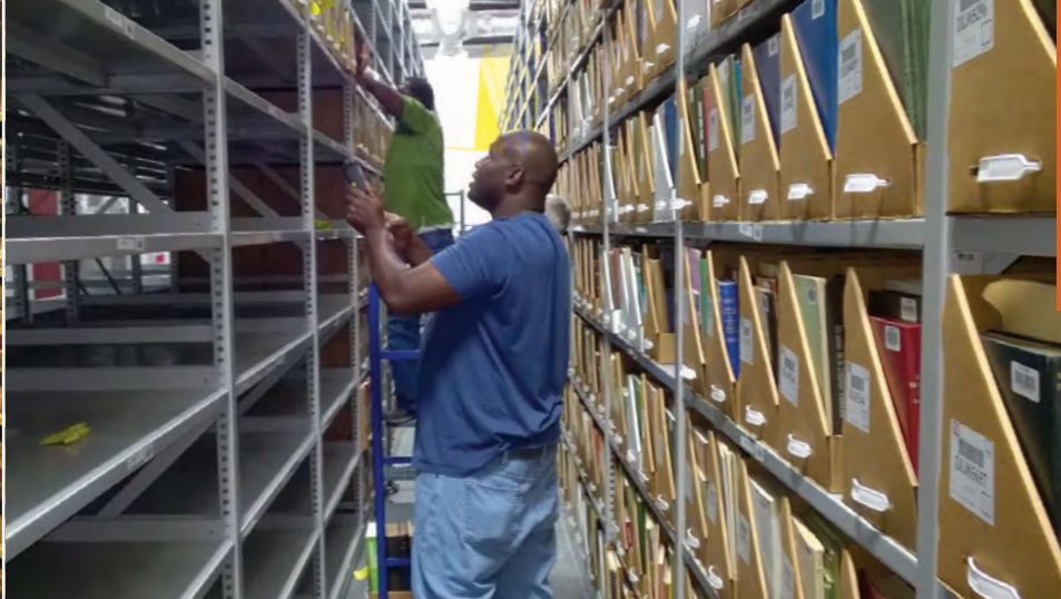
Fig. 6 “Lighting” new high density shelves at ALF in 2018. Each shelf has a unique barcode applied which is then scanned into the software. When a book is requested, the software tells staff exactly which shelf the item is on.
