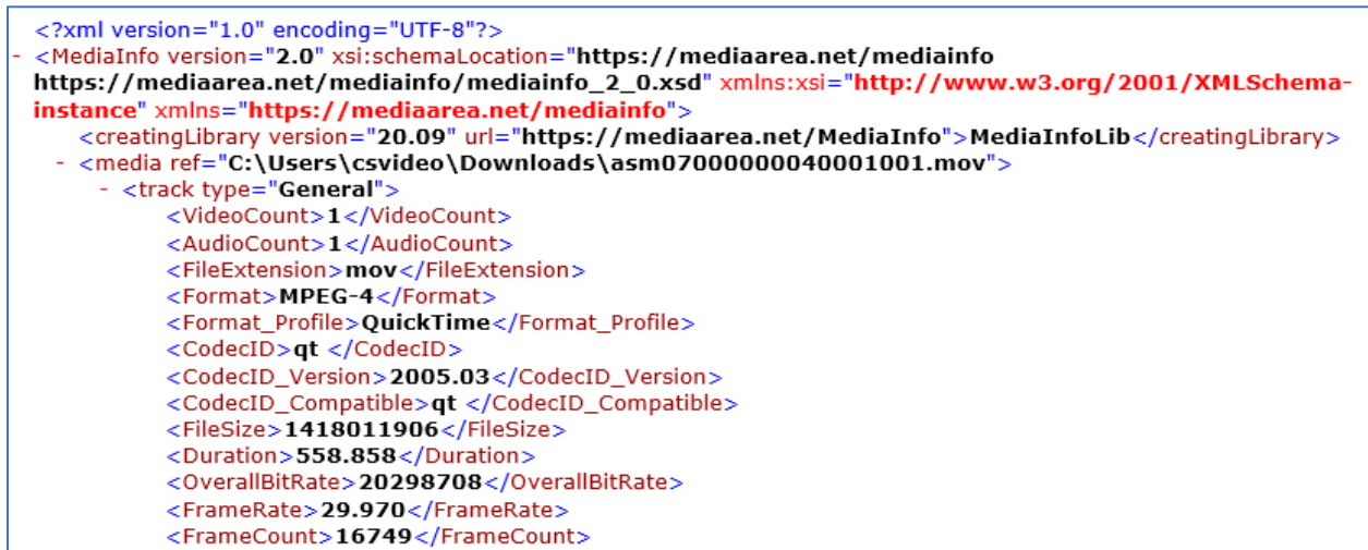
Figure 8. Example of a portion of an XML document which MediaInfo created from a video file.
