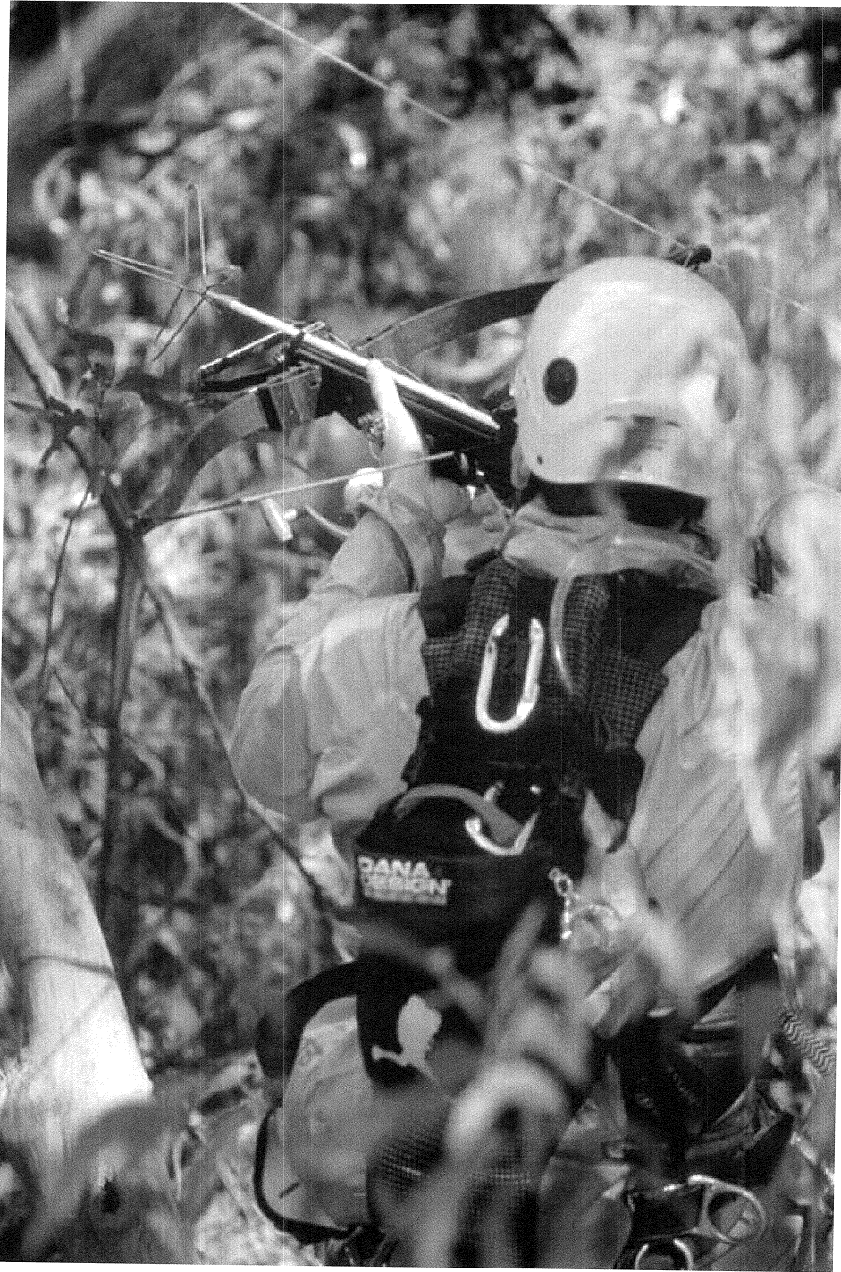
FIGURE 1. A retrieval bolt being fired at a throw bag line in an adjacent tree. Photograph courtesy of Bill Hatcher Photography.
