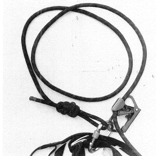
FIGURE 2. The waist assembly, attached to the sit-harness.
