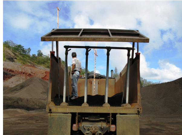
Fig. 5. Modified steam-delivery system in dump truck bed at the volcanic cinder mining site.
