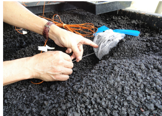
Fig. 2. Inserting thermocouple probes into Rotylenchulus reniformis inoculated large pore mesh cinder packet.
