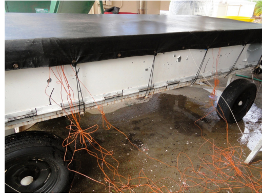
Fig. 1. Soil cart used for small scale steam sterilization of a volcanic cinder medium.
