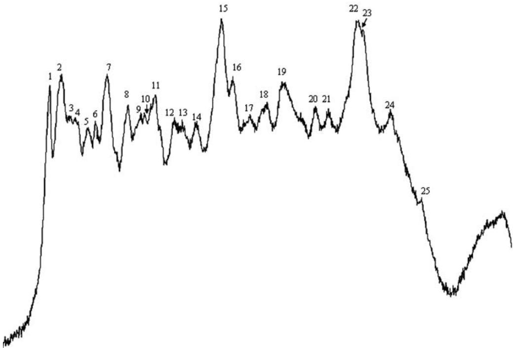
Fig. 2. Densitometry scan of population HG Type 1.2.3.4.5.6.7 (LY1) proteins from a SDS-PAGE gel. Molecular weight distribution from 202 to 47 kDa.
