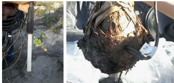
Fig. 1. PROB-107 sensor used to measure the internal temperature of banana rhizomes by embedding the temperature probe in rhizome tissue.
