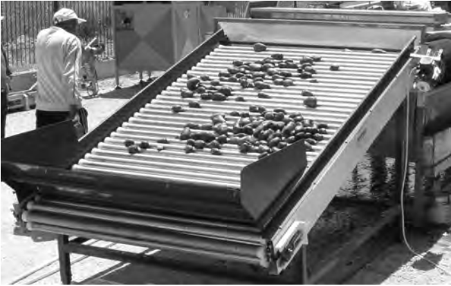
Fig. 1. The first component of the washing/brushing plant: the inclined delivery elevator.
