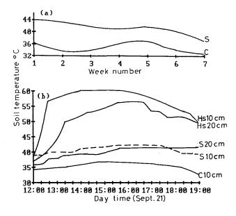
Fig. 1 - Effect of (a) solarization with black plastic (S) on soil temperature at 10 cm depth compared with non-covered control (C), and (b) solar hot water treatment of solarized soil (Hs) on soil temperature at two depths compared with solarization (S) or noncovered control (C) as recorded for 7 hours starting 12 a.m. on Sept. 21, 20 minutes after the beginning of hot application.
