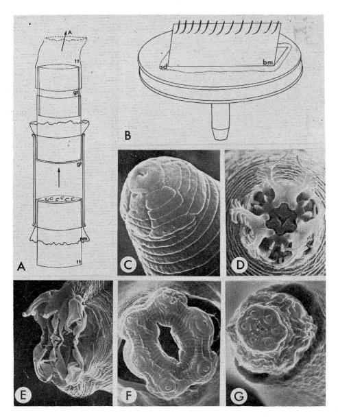
Fig. 1 - A: Processing chamber (McClure and Stowell, 1978) with syringe connected from A. Arrows indicate the direction fluids are drawn through the chamber towards the barrel of the syringe; gt = glass tubing; tt = teflon tubing; nm = nylon mesh. B: Stub prepared for nematode examination; bm = brass mount; sd = silver dag. C - G, face views. C: Scutellonema brachyurum. D: Acroboles complexus. E: Tylocephalus auriculatus. F: Aporcelaimellus sp. G: Tylencholaimellus sp.
