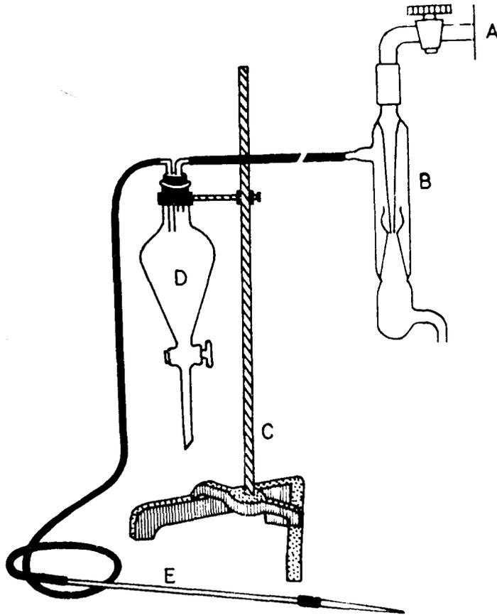
Fig. 1 - Diagram of the apparatus used for picking up of nematodes. A: water tap; B: aspirator; C: retort stand; D: separating funnel and E: glass tube with fine jet.
