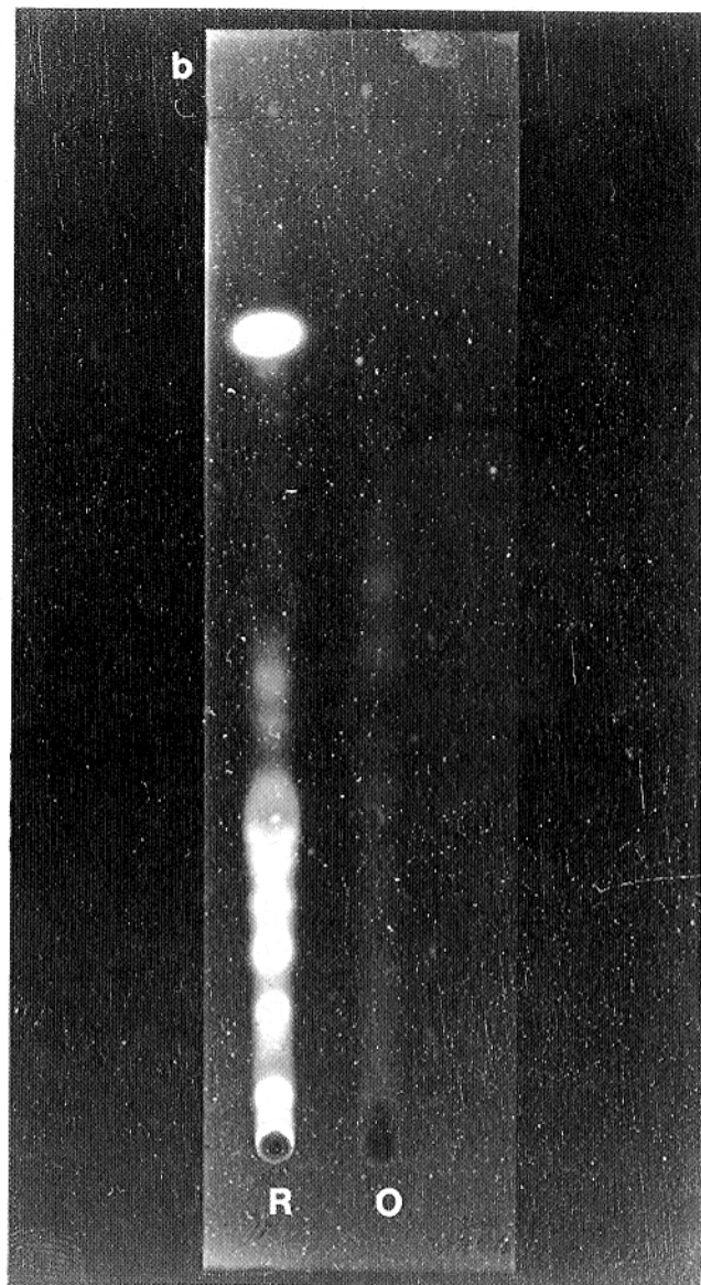
Fig. 3 - Thin layer chromatography (TLC) of a red pigment (R) produced by V. subblasporium (isolate 10) and oosporein (O), a red pigment produced by V. psalliotae , in toluene/ethyl acetate/formic acid (5:4:1, v/v/v) developed for 45 min. (a); same TLC plate under UV light (b).
