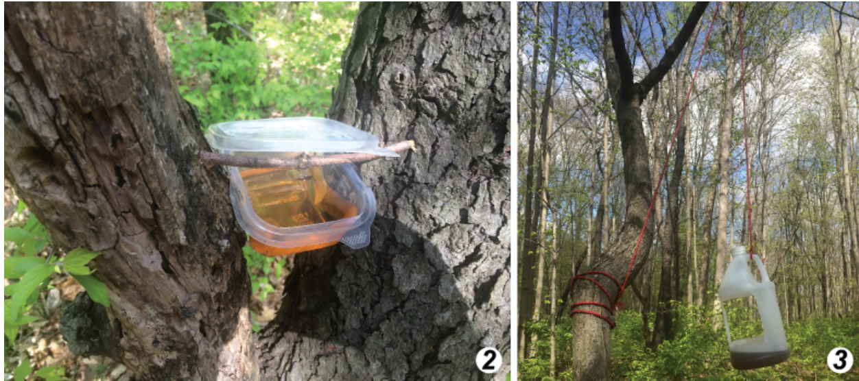
Figures 2–3. Examples of trap designs. 2) Plastic “jug” trap baited with fermenting mixture hung from tree branch in an open wooded area. 3) Plastic “boat” trap baited with apple cider vinegar placed in the crotch of a large tree. The lid is propped open to allow attractant to spread but still shield the container from rain.
