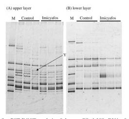
FIG. 3. PCR-DGGE analysis of the amplified 18S rDNA of nematodes from upper (0-10 cm depth) and lower layer (10-30 cm depth) of soil 91 d after treatment, 2008. M: marker lane. Y: band that disappeared in the imicyafos treatment.
