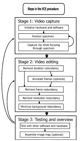
FIG. 1. Overview of the main steps in the VCE procedure.
