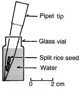
FIG. 1. Diagram of the simple extraction apparatus used for obtaining *Aphelenchoides besseyi* from an *Oryza sativa* seed.
