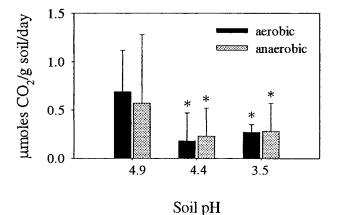
FIG. 2. CO<sub>2</sub> evolved over 7 days as a function of soil pH under aerobic and anaerobic soil atmospheres. Soil was amended with HCI to adjust the pH. Values are means  $\pm$  SD (n = 10). (\*) Different from control ( $P \le 0.05$ ).
