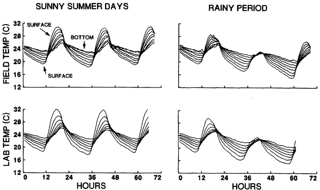
FIG. 3. Soil temperature gradients measured 5–25 cm deep in a cotton field during late summer in eastern Texas and laboratory simulations of those gradients. Thermocouples were positioned at 2.5-cm intervals in the field and at 3.3-cm intervals in the laboratory. Because the uppermost thermocouple in the field malfunctioned during these measurements, the corresponding field temperatures are not given.
