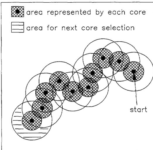
FIG. 1. Sampling pattern with spatial constraints; each core is selected at random from an area between two circles, one of radius  $d_{min}$  and one of radius  $d_{max}$ , centered on the location of the previous core. The area available for each core excludes any overlap of the sampling area with the sampling areas of any previous core.
