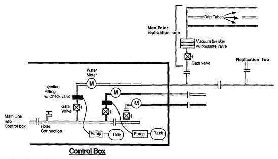
FIG. 5. Detailed schematic of control box connection to treatment manifold for nematicide application through drip irrigation in research on Hawaiian pineapple. Each manifold serves one replication, with each replication consisting of three beds, one drip tube per bed.
