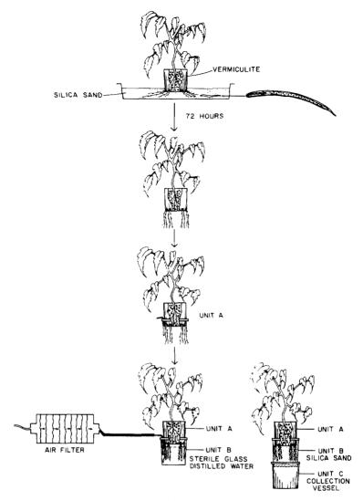
FIG. 3. Diagram of the apparatus designed for long-term production and recovery of root exudates from *Meloidogyne incognita*-infected tomato roots. Plants in plastic pots (Unit A) were set in sand and extending roots were inoculated with nematodes, removed from the sand, washed, and placed in a second plastic container (Unit B). A third container (Unit C) acted as a collection vessel for root exudates.
