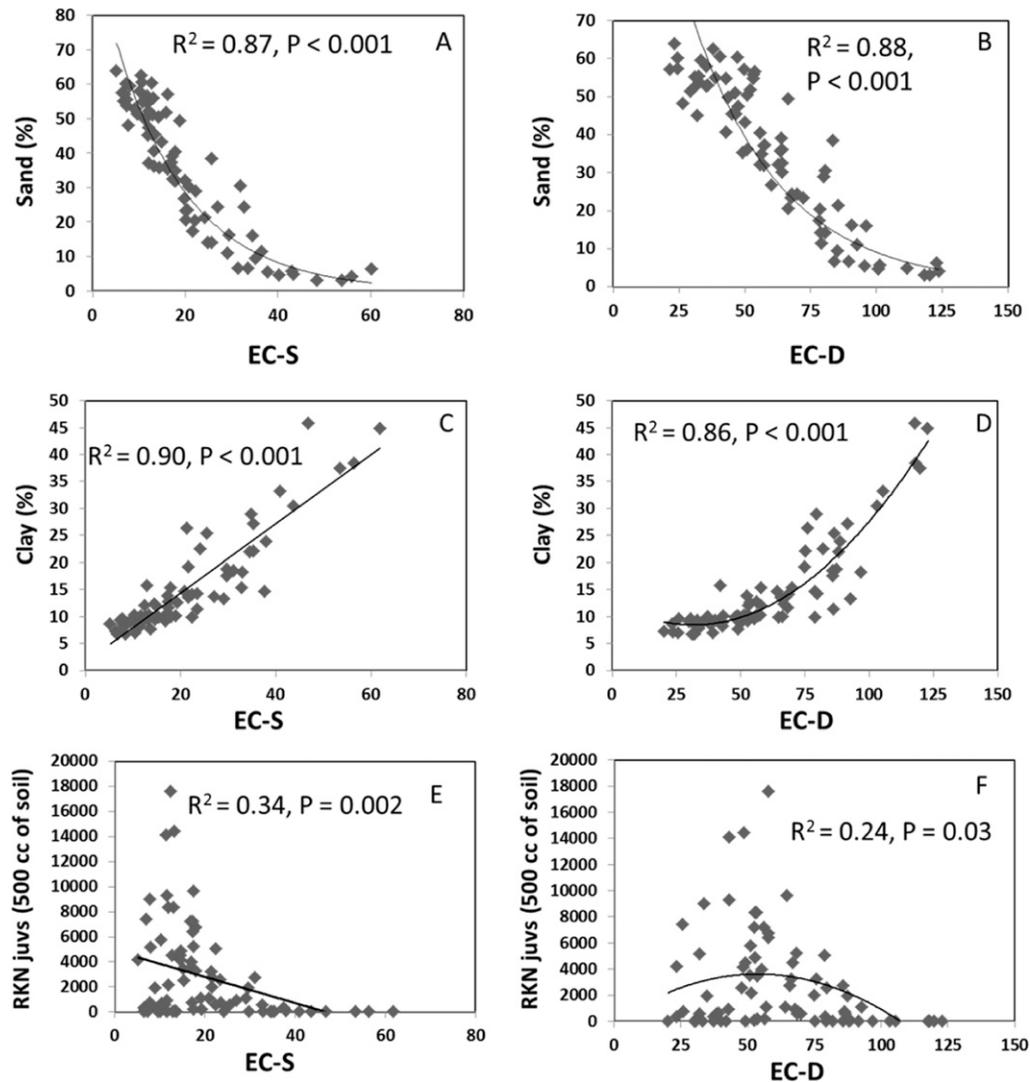
FIG. 2. Panels illustrate the relationship between the content of sand in the upper 20 cm of soil and (A) EC-S ( $EC_{a\text{-shallow}}$ ) and (B) EC-D ( $EC_{a\text{-deep}}$ ); the relationship between clay content in the upper 20 cm of soil and (C) EC-S and (D) EC-D; and the relationship between (E) EC-S and (F) EC-D and numbers of *Meloidogyne incognita* second-stage juveniles (RKN juvs/500 cc of soil). The experiment was conducted at Northeast Research Station, St. Joseph, LA, in 2003.
