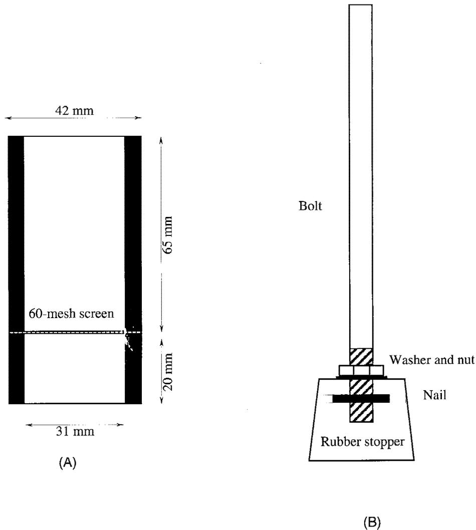
FIG. 1. A) Longitudinal section of a cyst-crushing chamber built with two pieces of PVC pipe with 60-mesh (250- $\mu$ m pore size) screen between them. B) Plunger constructed with a no. 6 rubber stopper and a 130-mm-long bolt.
