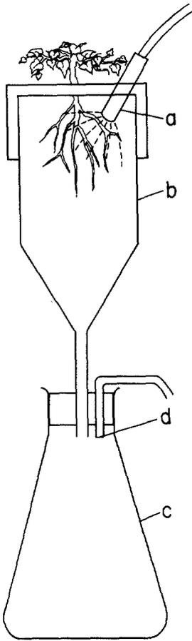
FIG. 1. Extraction apparatus for *Meloidogyne* juveniles hatching from egg masses on growing plants. a = nozzle delivering water at a rate of 2.38 liters/hour for 8 seconds every 10 minutes; b = light-proof chamber; c = collection flask; d = 45- $\mu$ m-opening sieve on drainage port.
