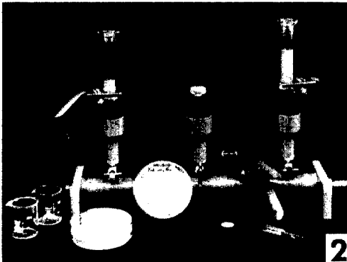
FIG. 2. Equipment used for collecting residues on filter paper disks for placement onto agar plates.
