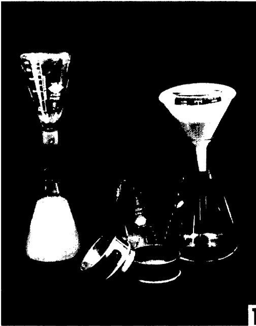
FIG. 1. Equipment for sieving and decanting soil samples after agitation in joined flasks.
