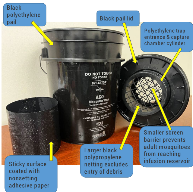
Figure 1. AGO trap consists of the black polyethylene pail with lid and a sticky surface coated to adhesive paper for trapping of gravid females.
