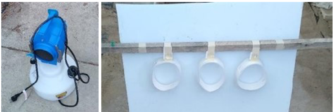
Figure 2: Portable ULV Sprayer and Field Cages (Blue board was not present during application and was used only for better contrast in the picture).
