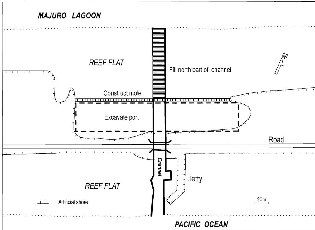
Figure 7. Recommendation of reforming present artificial channel crossing through reef flat into an access channel-port: to excavate a small port on reef flat north to the bridge and fill the channel north to the recommended port. Location in Figure 1.
