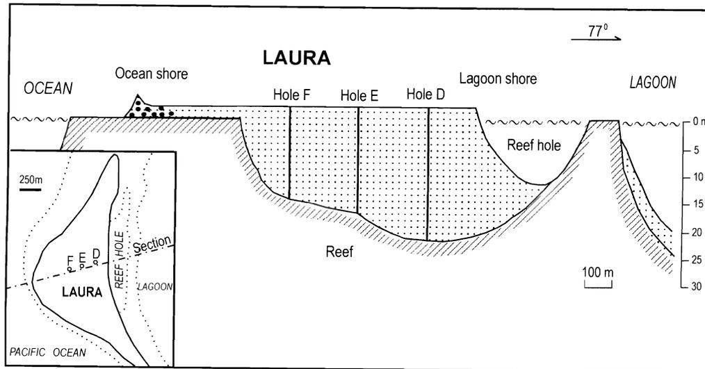
Figure 2. A cross-section from ocean to lagoon in middle Laura, showing that the original reef hole has been mostly filled up by sand transported from the lagoon coast of the south rim. The data of the drill holes are from ANTHONY and PERTESON (1987). The surface and shallow subsurface sediments are based on field survey and some shallow drill holes. Location in Figure 1.
