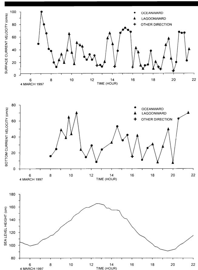
Figure 6. Surface current velocity (upper), bottom current velocity (middle) at the artificial channel crossing through the reef flat between ocean and lagoon, and tidal level (lower) in Majuro Atoll. The tide data are from the Sea Level Center, of the University of Hawaii.
