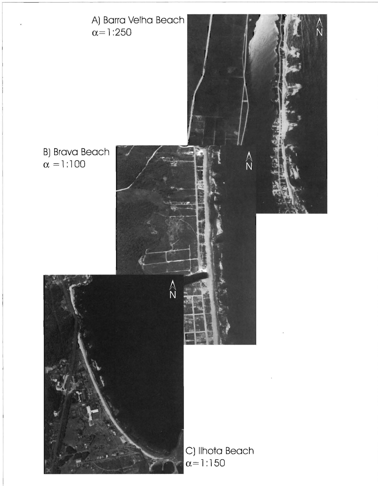
Figure 11. Intermediate beaches with different types of bar system at: (a) Barra Velha beach; (b) Brava beach and (c) Ilhota beach (original scale 1:12,500).
