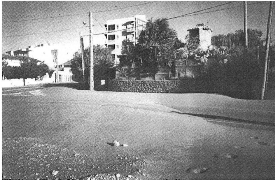
Figure 7. Sand accumulation in the street and surrounding a house immediately inland from the beach, total volume at this site is approximately 45 m 3 , following a severe Tramontana event.
