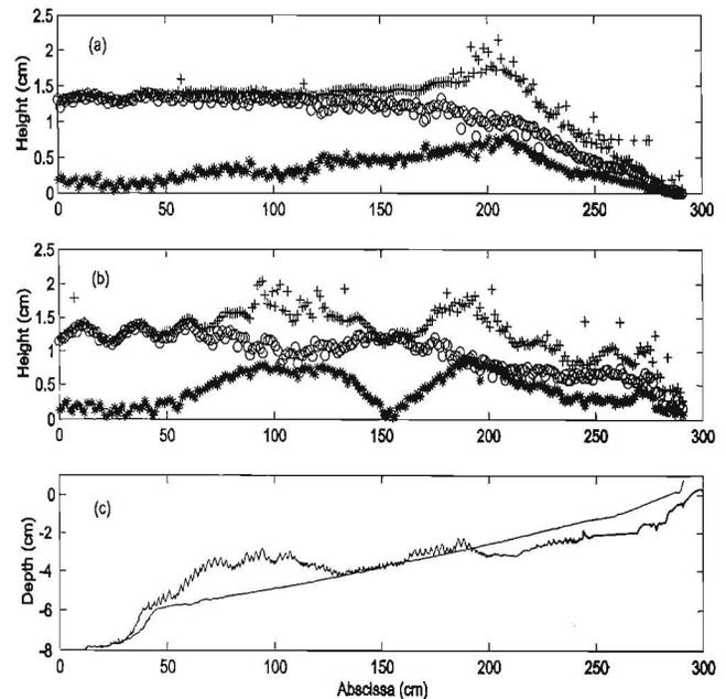
Figure 7. Envelope of the initial wave (a), and final (b) and bathymetric profile (c) after 4660 min of wave action under breaking conditions ( $H_0 = 1.9$  cm,  $D_1 = 0.08$  mm).
