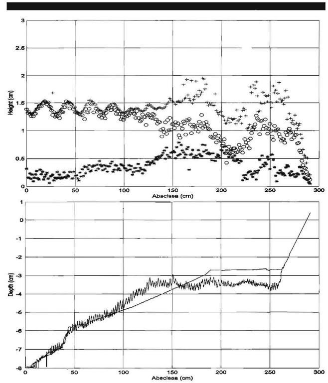
Figure 9. (a) Envelope of (+) the total wave and of (O) first and (\*) second harmonics at 1320 min, above (b) the initial bathymetric profile (---) and at 1320 min (—) ( $H_0 = 1.6$  cm and  $D_1 = 80$   $\mu$ m).
