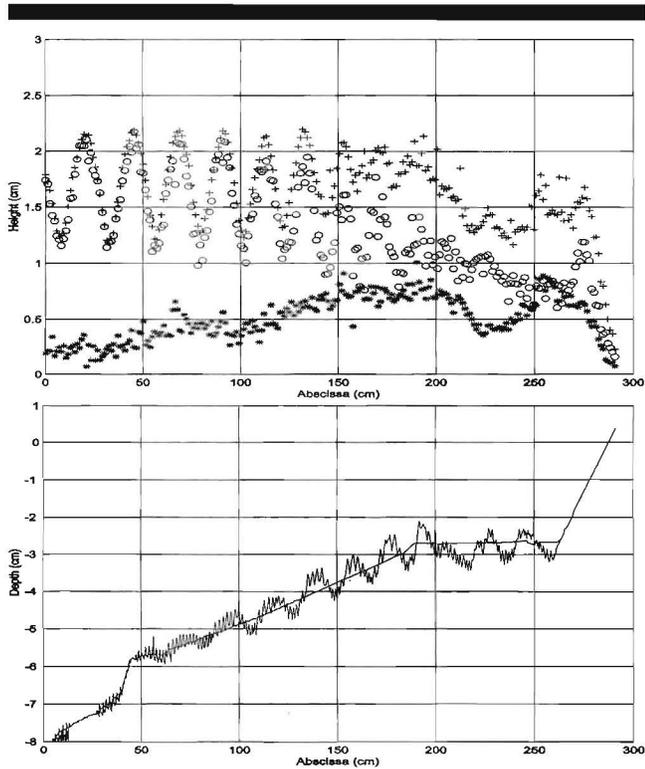
Figure 8. (a) Envelope of (+) the total wave and of (O) first and (\*) second harmonics at 60 min, above (b) the initial bathymetric profile (---) and at 60 min (—) ( $H_0 = 1.6$  cm and  $D_1 = 80$   $\mu$ m).
