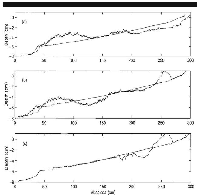
Figure 5. Final bathymetric profiles under breaking conditions for  $D_1 = 0.08$  mm and  $\psi_{D_1} = 34.3$  (suspended load) (a),  $D_2 = 0.12$  mm and  $\psi_{D_2} = 22.9$  (intermediate) (b) and  $D_3 = 0.20$  mm and  $\psi_{D_3} = 13.7$  (bedload) (c) ( $H_0 = 1.9$  cm,  $H_b = 2.5$  cm and  $h_b = 2.9$  cm).
