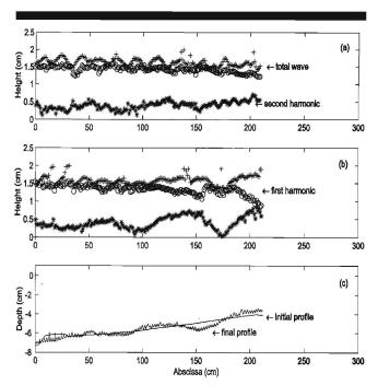
Figure 4. Envelope of the initial wave (a), final (b) and bathymetric profile (c) after 2660 min of wave action under non-breaking conditions ( $H_0 = 1.7 \text{ cm}$  and  $R_b < 0.05$ ,  $D_1 = 0.08 \text{ mm}$ ).
