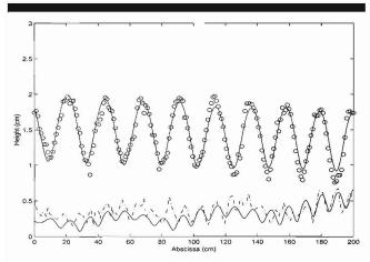
Figure 2. (case 1) Comparison of the envelope of both first and second harmonics for a gently sloping bottom and without any parasitic wave: (——) model, measurements ( $\bigcirc$ ) first harmonic, (---) second harmonic.
