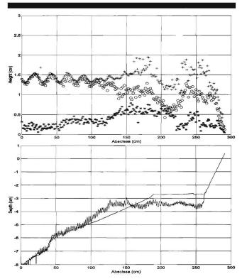
Figure 9. (a) Envelope of (+) the total wave and of ( $\bigcirc$ ) first and (\*) second harmonics at 1320 min, above (b) the initial bathymetric profile (---) and at 1320 min ( $\longrightarrow$ ) ( $H_0=1.6$  cm and  $D_1=80$   $\mu$ m.
