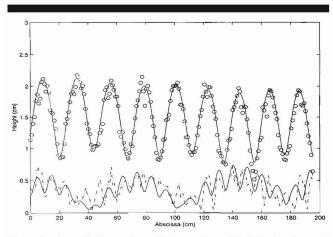
Figure 3. (case 2) Comparison of the envelope of both first and second harmonics for a gently sloping bottom and without any parasitic wave: (——) model, measurements ( $\bigcirc$ ) first harmonic, (---) second harmonic.
