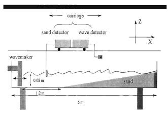
Figure 1. Sketch of the wave flume in the breaking configuration.
