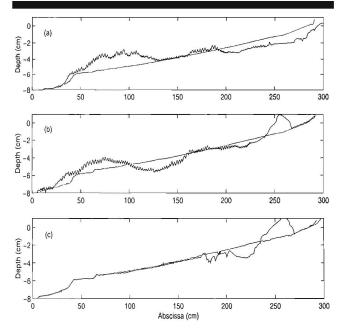
Figure 5. Final bathymetric profiles under breaking conditions for  $D_1=0.08$  mm and  $\psi_{D_1}=34.3$  (suspended load) (a),  $D_2=0.12$  mm and  $\psi_{D_2}=22.9$  (intermediate) (b) and  $D_3=0.20$  mm and  $\psi_{D_3}=13.7$  (bedload) (c) ( $H_0=1.9$  cm,  $H_b=2.5$  cm and  $h_b=2.9$  cm).
