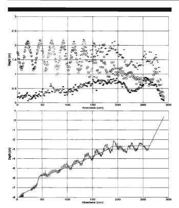
Figure 8. (a) Envelope of (+) the total wave and of ( $\bigcirc$ ) first and (\*) second harmonics at 60 min, above (b) the initial bathymetric profile (--) and at 60 min ( $\bigcirc$ ) ( $H_0 = 1.6$  cm and  $D_1 = 80$   $\mu$ m.
