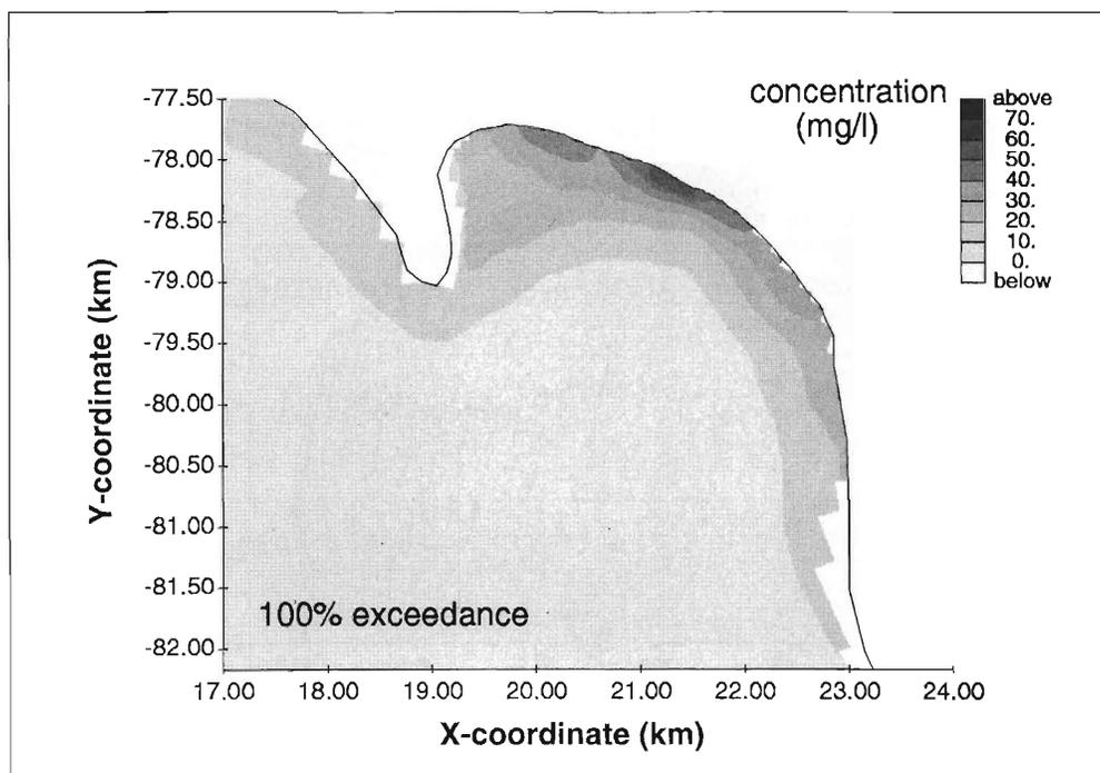
Figure 18. Predicted regions of exceedance of concentration thresholds (in mg/l indicated on the shaded scale) for May 1997.
