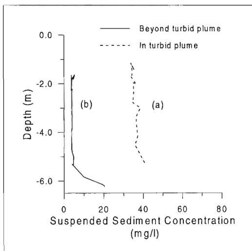
Figure 14. Suspended sediment concentrations measured (a) within and (b) beyond the limits of a turbid plume.
