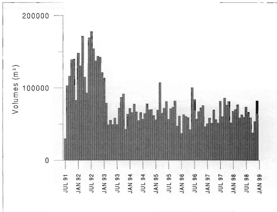
Figure 5. Monthly volumes of mine tailings sediment discharged onto the beach.
