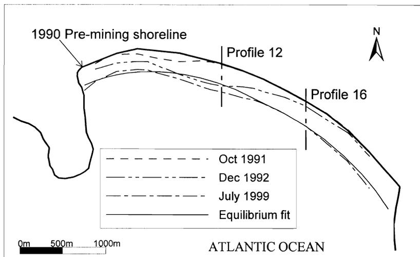
Figure 8. Measured shorelines (MSL-0 m contours) and a prediction of the equilibrium bay configuration in July 1999.
