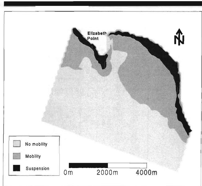
Figure 15. Predicted regions of sediment mobility and suspension ( $d_{50} = 300 \mu\text{m}$ , offshore wave conditions  $H_{m0} = 2$  m,  $T_p = 8$  s, wave direction = south).
