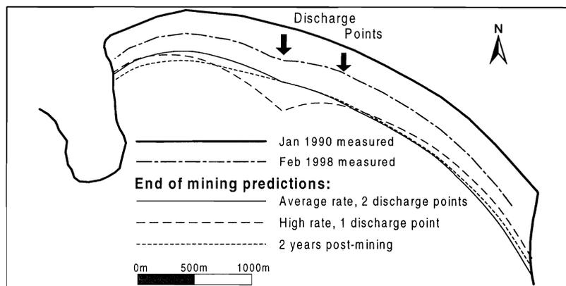
Figure 12. Predictions of the shoreline configuration after discharge of 15 million m<sup>3</sup> of sediment, and the situation 2 years later.
