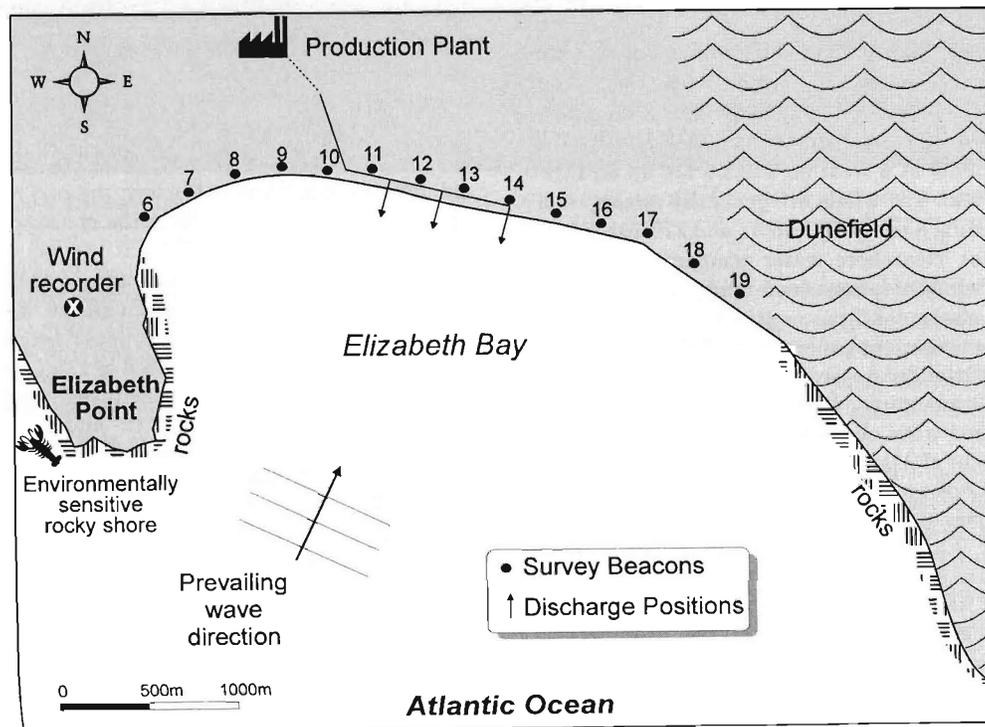
Figure 2. Schematic plan of Elizabeth Bay, showing sediment discharge locations.
