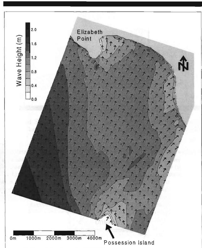
Figure 3. Simulated wave refraction pattern ( $H_{m0} = 2\text{ m}$ ,  $T_p = 8\text{ s}$ ,  $\Theta = 180^\circ\text{ N}$ ).
