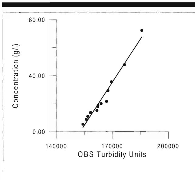
Figure 6. Optical Backscatter Sensor calibration result.
