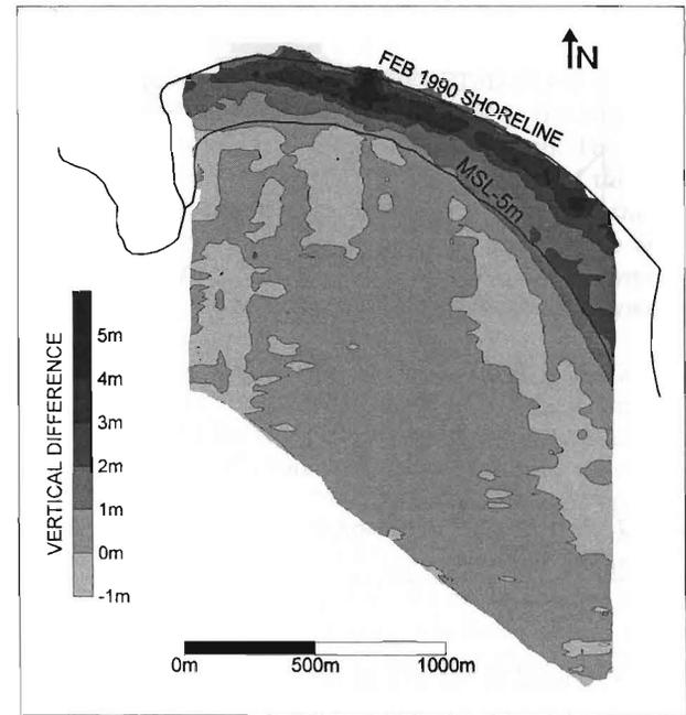
Figure 10. Bathymetry difference chart showing the distribution of vertical differences (as indicated by the shaded scale) between the measured surfaces of May 1997 and February 1990.
