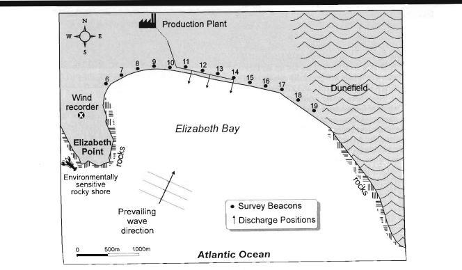
Figure 2. Schematic plan of Elizabeth Bay, showing sediment discharge locations.
