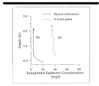
Figure 14. Suspended sediment concentrations measured (a) within and (b) beyond the limits of a turbid plume.
