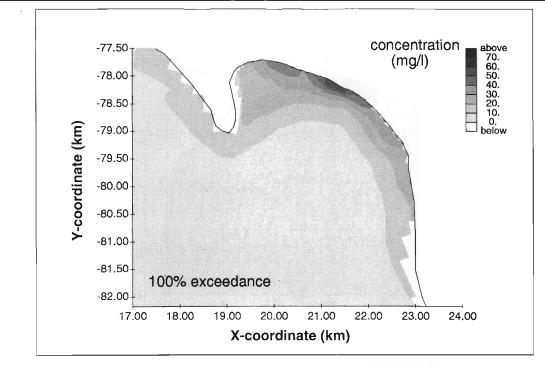
Figure 18. Predicted regions of exceedance of concentration thresholds (in mg/l indicated on the shaded scale) for May 1997.
