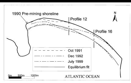
Figure 8. Measured shorelines (MSL-0 m contours) and a prediction of the equilibrium bay configuration in July 1999.
