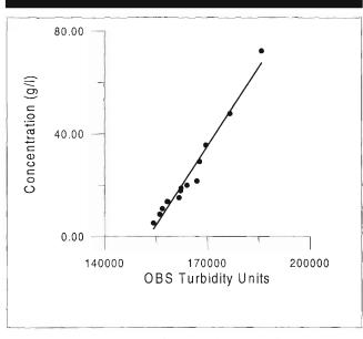
Figure 6. Optical Backscatter Sensor calibration result.
