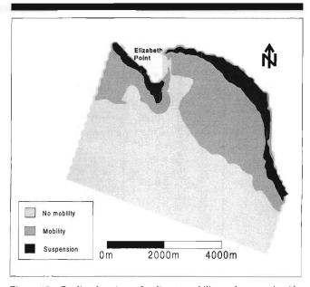
Figure 15. Predicted regions of sediment mobility and suspension ( $d_{so}$  = 300 µm, offshore wave conditions  $H_{mo}$  = 2 m,  $T_{p}$  = 8 s, wave direction = south).
