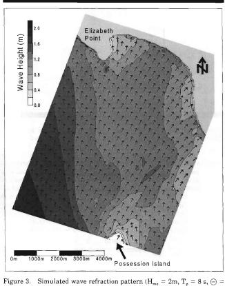
Figure 3. Simulated wave refraction pattern ( $H_{mo} = 2m$ ,  $T_p = 8 s$ ,  $\bigcirc = 180^{\circ}$  N).
