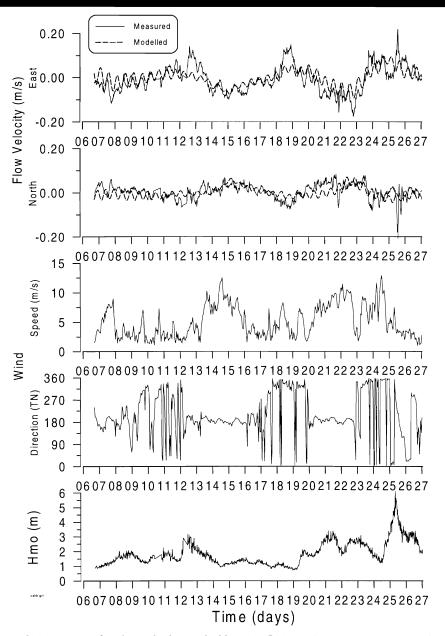
Figure 16. Modelled current velocities compared to observed velocities for May 1997 (Position of measurement, Figure 7, depth of measurement = 9 m, water depth = 20 m), and associated wind and wave conditions.
