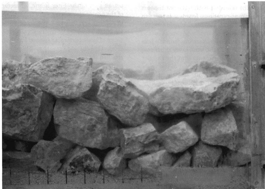
Figure 5. Test Section During the Experiment (Showing Water Surface Level Decline in the Direction of Flow).
