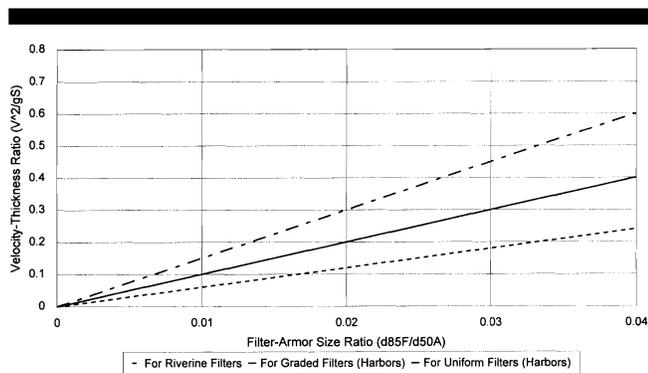
Figure 10. Relationship between Velocity-Thickness Ratio and Filter-Armor Size Ratio.
