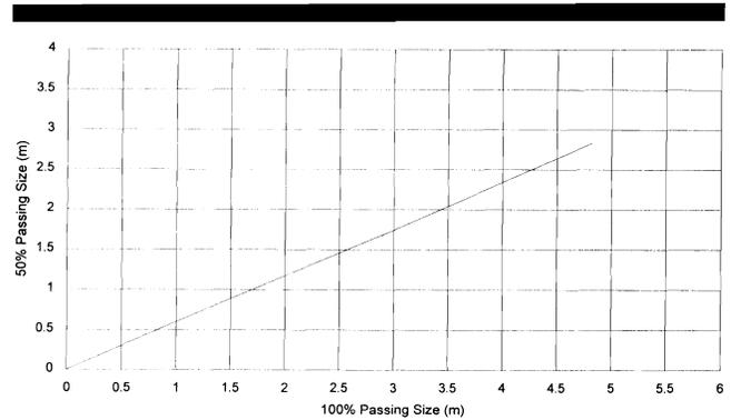
Figure 8. Relationship between 50% Passing Size and 100% Passing Size for Filters.
