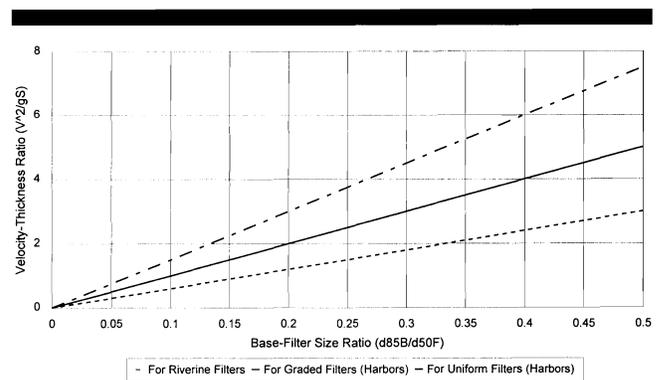
Figure 9. Relationship between Velocity-Thickness Ratio and Base-Filter Size Ratio.
