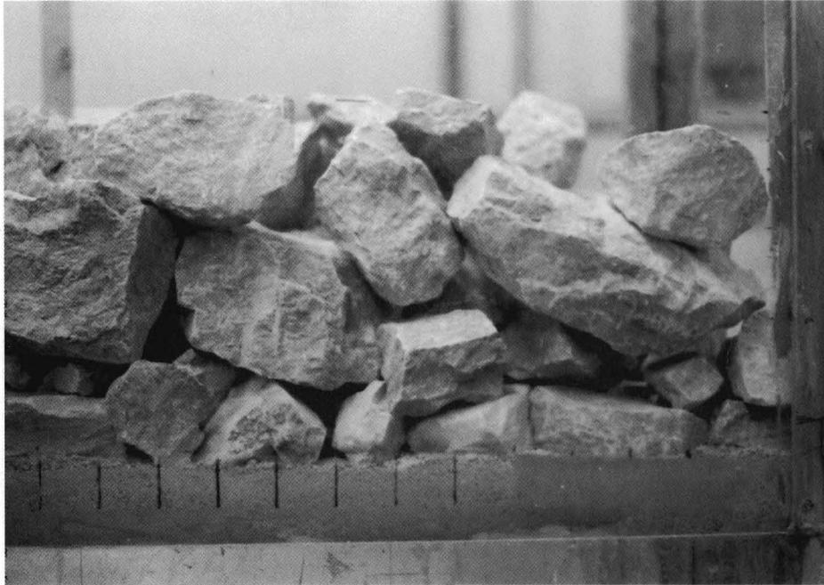
Figure 4. Completed Test Section (With Final Layer of 4-8 inch Armor Layer).
