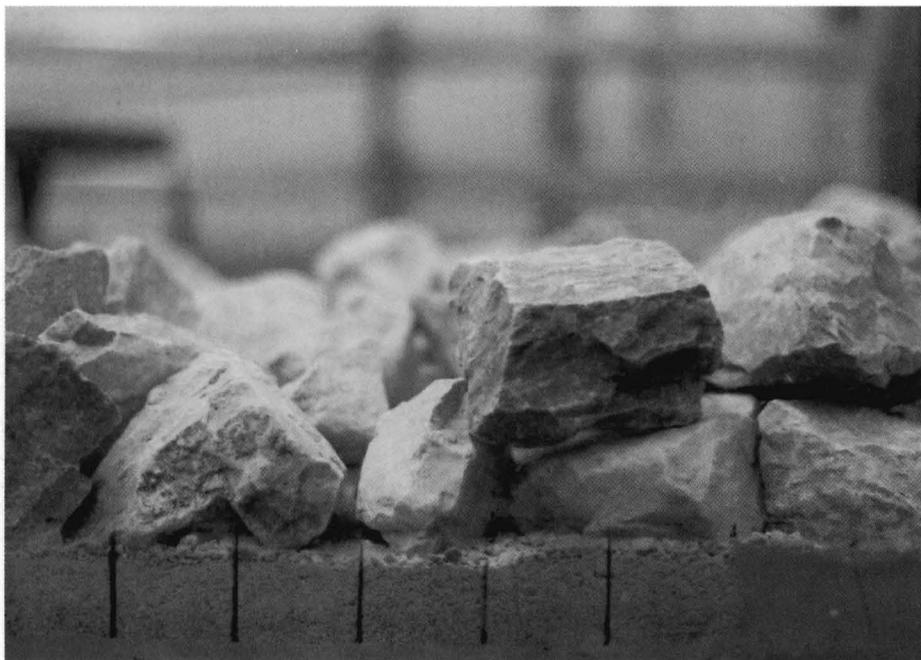
Figure 3. Intermediate Stage of Test Section Construction (Placement of 4 inches of 2–4 inch Armor over Sand Isolation Layer).
