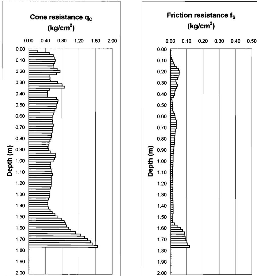
Figure 4. Results of cone resistance and friction resistance from a penetrometer test in a Mississippi delta coastal marsh. The strong increase in the two parameters at 1.5 m is due to the presence of a clay layer associated with an old channel of the Mississippi River. See text for discussion.
