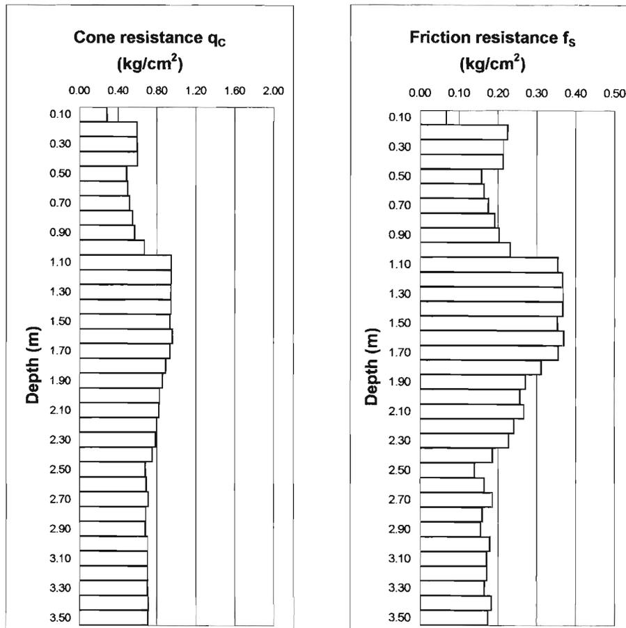
Figure 3. Results of cone resistance and friction resistance from a penetrometer test at Punta Vecia in Venice Lagoon. The strong increase between 0.9 to 2.1 m is due to the presence of a layer with a higher sand content. See text for discussion.
