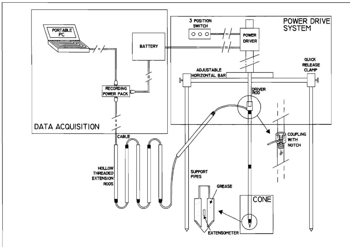
Figure 1. Diagram of the Portable Electric Penetrometer showing the three main components of the instrument: the power drive system, the cone and the data acquisition system.
