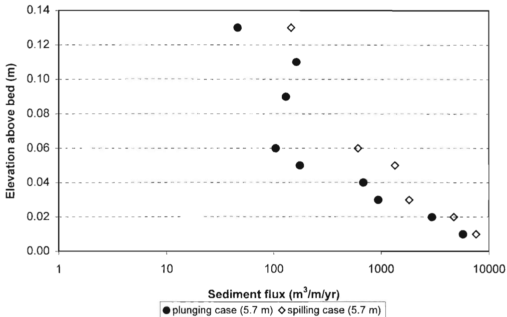
Figure 12. Sediment-flux profiles in the mid-surf zone. Numbers in the legends denote distance to the still-water shoreline.
