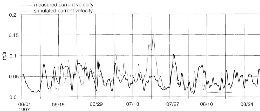
Figure 3. Comparison between measured and modelled bottom current velocities at ODAS Tonne.
