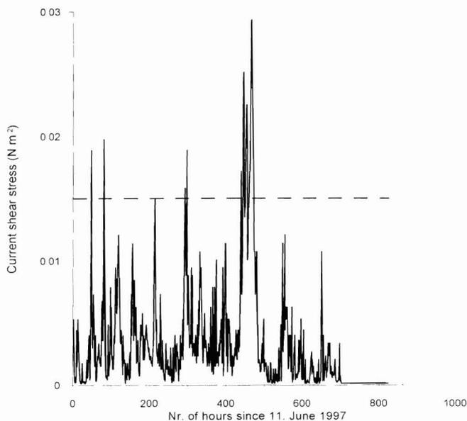
Figure 10. Current induced shear stress at ODAS Tonne from 11 June to 19 August 1997. Threshold shear stress for resuspension is shown with hatched line.
