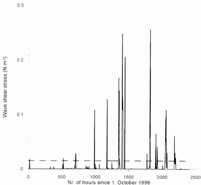
Figure 5. Wave-induced shear stresses at the bottom at ODAS Tonne. Threshold shear stress for resuspension is shown with hatched line.
