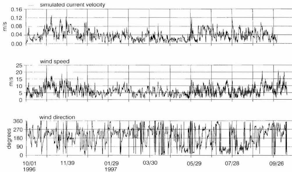
Figure 4. Wind speed and direction from HIRLAM data compared to simulated yearly variation in bottom current velocities at ODAS Tonne.
