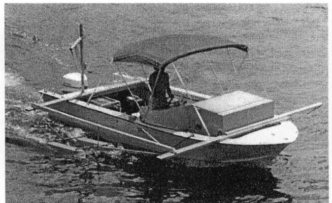
Subbottom seismic reflection data is gathered using an EG&G Uniboom. The data at this site was used to identify a zone of paleokarst collapse along the planned route of a new bridge in the Florida Keys.
