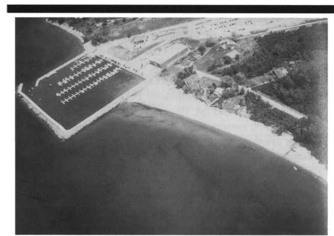
Figure 7. The Soft Harbor Marina, Lake Erie, leeside erosion (RAYMOND and TAYLOR, J. Coastal Res. Special Issue No. 26, 1998, pp.).
