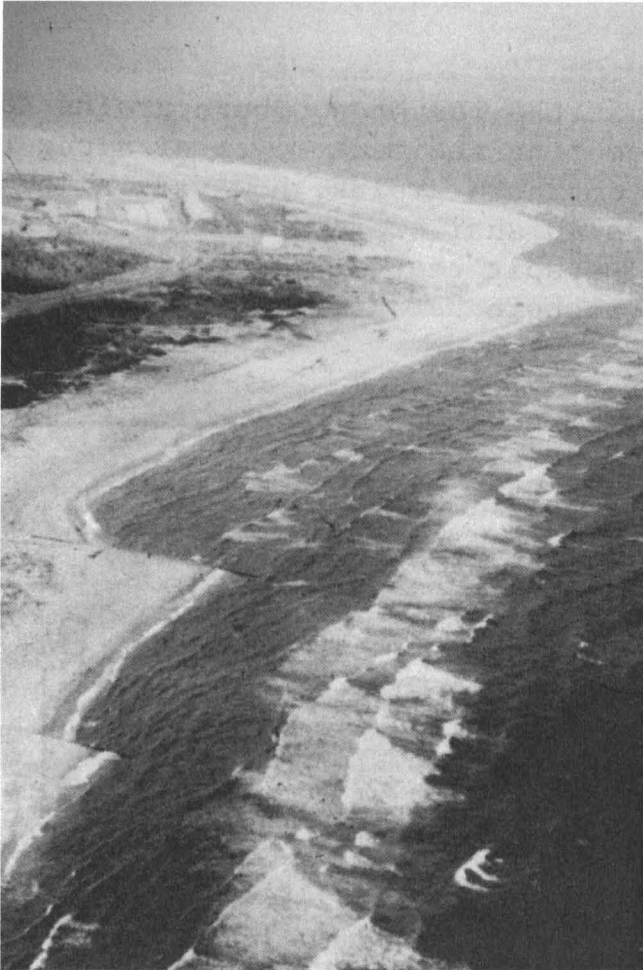
Figure 1. The northern part of Sandy Hook, New Jersey, demonstrating groin-effect and attachment of bar to shore (ALLEN and NORDSTROM, 1977).
