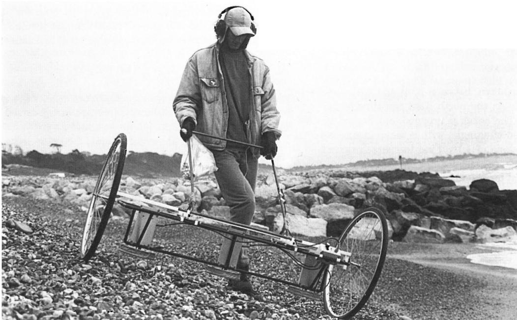
Plate 2. One coil (a) and 3-coil (b) detectors used for the recovery of the transmitting pebble tracers.
