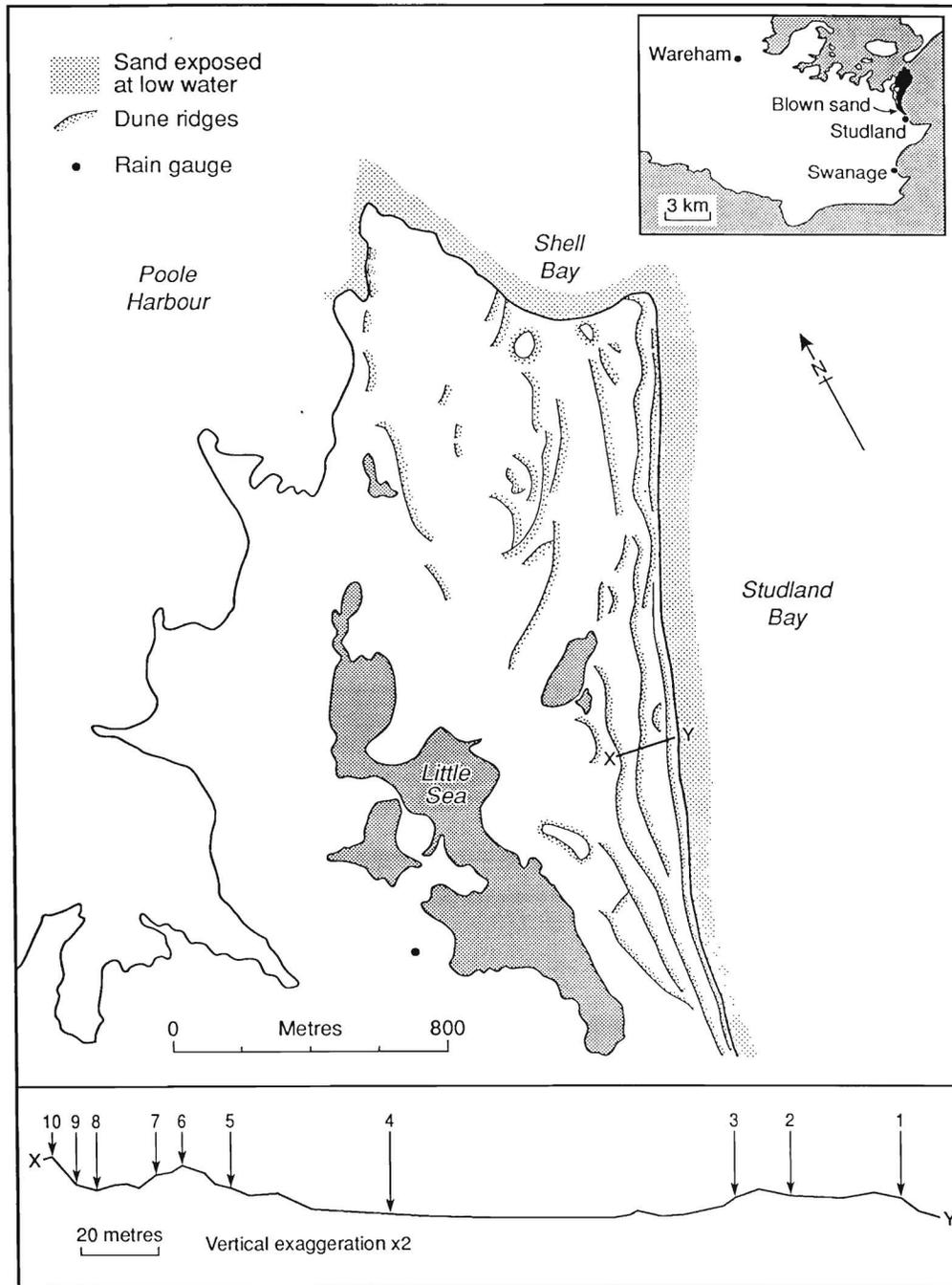
Figure 1. The dune system at Studland showing the location of the capacitance probe access tubes (1-10) across three of the dune ridges.
