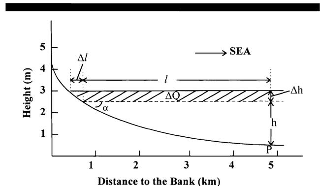
Figure 5. Diagram for the derivation of the interrelationship between  $V$ ,  $R$  and  $tg\alpha$ .
