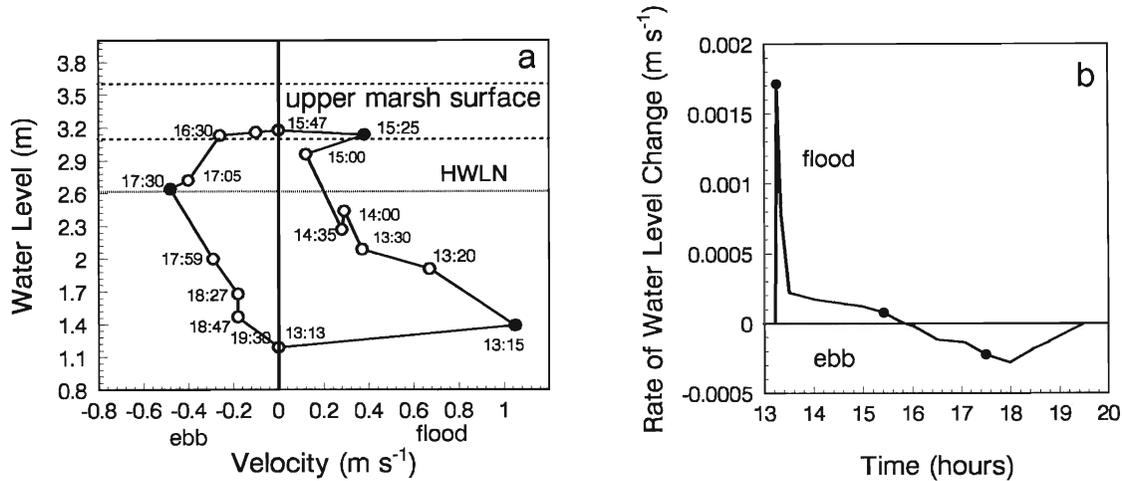
Figure 3. The velocity-water level relationship (a) and the rate of water level changes (b), measured in Fengche Creek, 11th September, 1979 (in the figure, HWLN denotes high water level on neaps).
