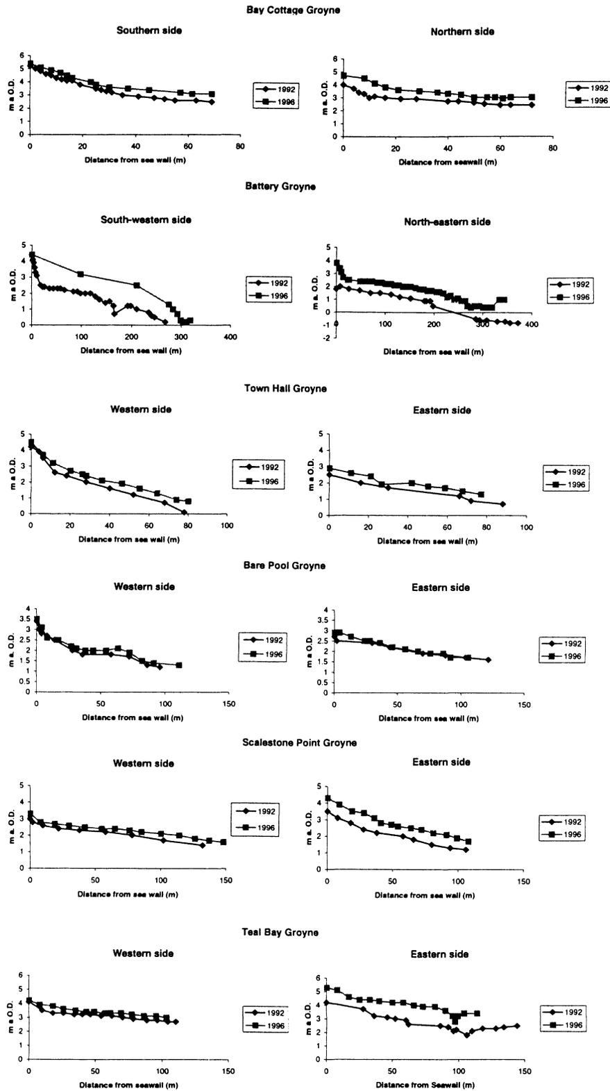
Figure 5. Sediment accretion between 1992 and 1996 for each of the six groynes studied.
