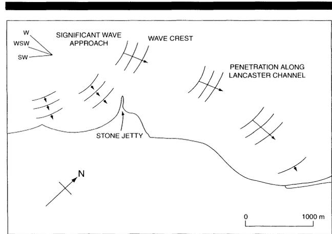
Figure 2. General wave climate along the Morecambe Frontage. (Modified from SMP 1990).
