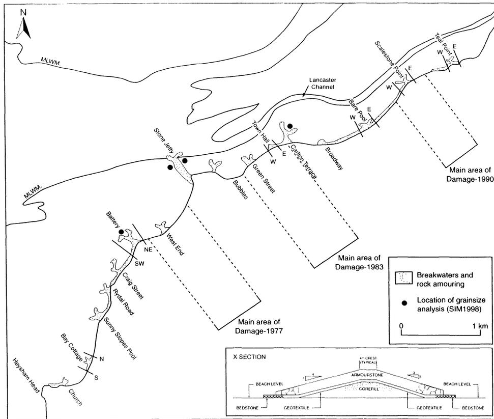
Figure 3. The Fish-tail groyne scheme along the Morecambe frontage showing areas of storm damage in 1977, 1983, and 1990 and approximate position of low water channels. For each of the six groynes studied, transects are marked and labelled according to their description in the text. Locations of sediment grain-size analysis are marked with '●'.
