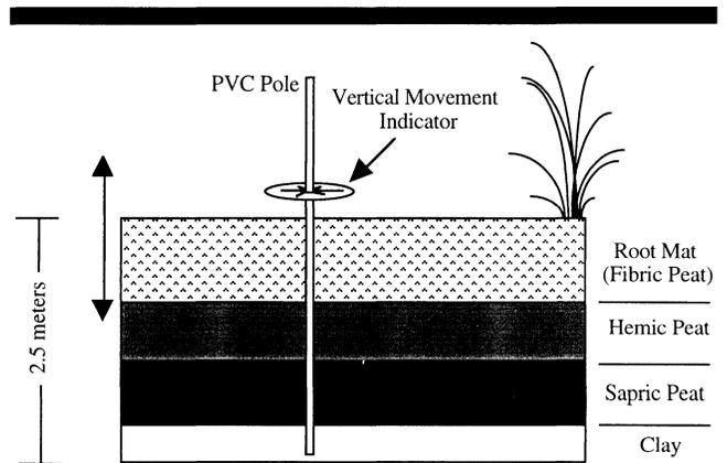
Figure 2. Diagram of a vertical movement indicator used to measure the maximum upward movement of the marsh surface. A buoyant marsh mat moves the disk upward, thereafter the disk holds its position until an event of greater movement. The PVC pole is driven through the peat to a firm substrate. Increasing stages of peat decomposition with depth below the root mat were evident in the oligohaline marsh substrates of this study.
