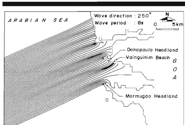
Figure 4. Wave refraction diagram for the waves of 8 s period coming from 250 w.r.t. North.
