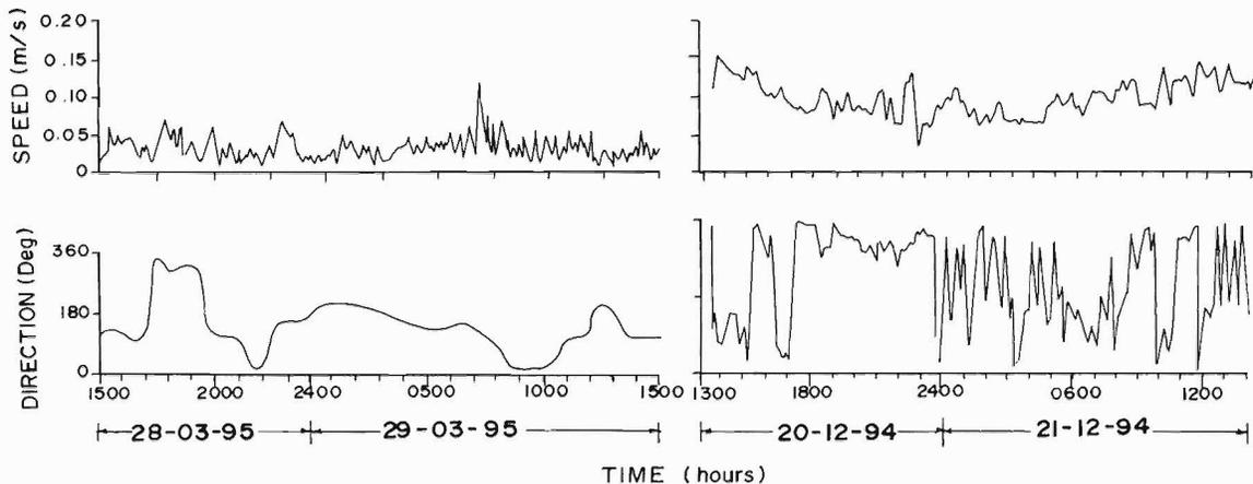
Figure 5. Variation of current speed and direction using S4 current meter at 3 m water depth.
