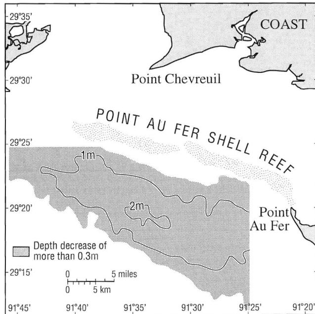
Figure 5. This figure illustrates the general thickness of "gelatinous muds" seaward of the Point Au Fer shell reef trend, interpreted as newly deposited Atchafalaya River sediment (modified from Thompson, 1951). Note that these deposits were approximately 2 m thick in the area of data collection just seaward of the Point Au Fer shell reef.
