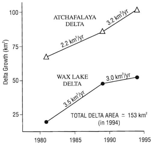
Figure 8. Growth of both the Atchafalaya and Wax Lake deltas measured in  $\text{km}^2$  above the  $-0.6$  m isobath. Measurements were made for 1981, 1989, and 1994. Rates of change are indicated in  $\text{km}^2/\text{yr}$  between the measurement years (modified from Majersky *et al.*, 1997).
