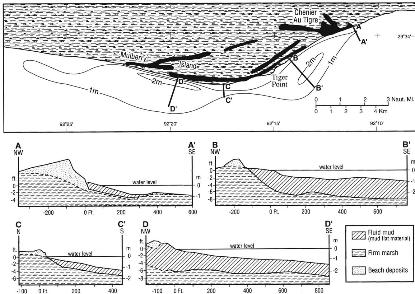
Figure 13. Map and selected cross sections showing the thicknesses of fluid mud deposits along the eastern chenier plain (modified from Morgan *et al.*, 1953). In the map view, distances from the shoreline have been exaggerated 9x for illustration purposes. Note that all cross sections except D-D' start at the shoreline in coarse-grained chenier ridge-beach deposits. At this time fluid mud from the Atchafalaya diversion was just starting to prograde the eastern chenier plain coast.
