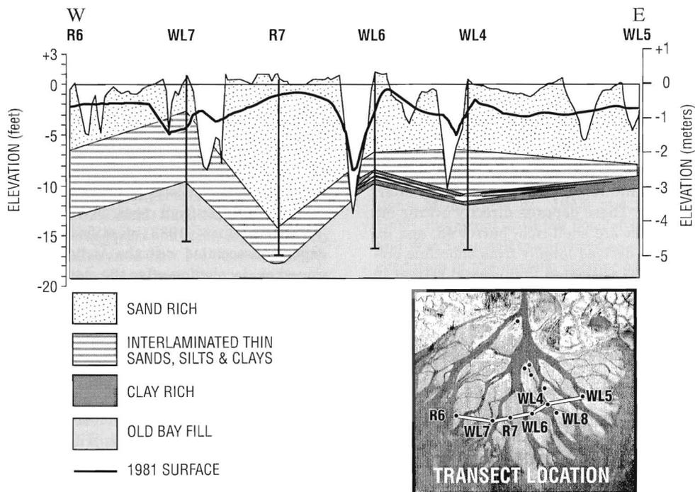
Figure 11. An interpretive strike-oriented cross section of the Wax Lake delta as compiled from vibracores (modified from Roberts *et al.*, 1997). Note the dominance of sand-rich facies and the thin fine-grained base of this delta.
