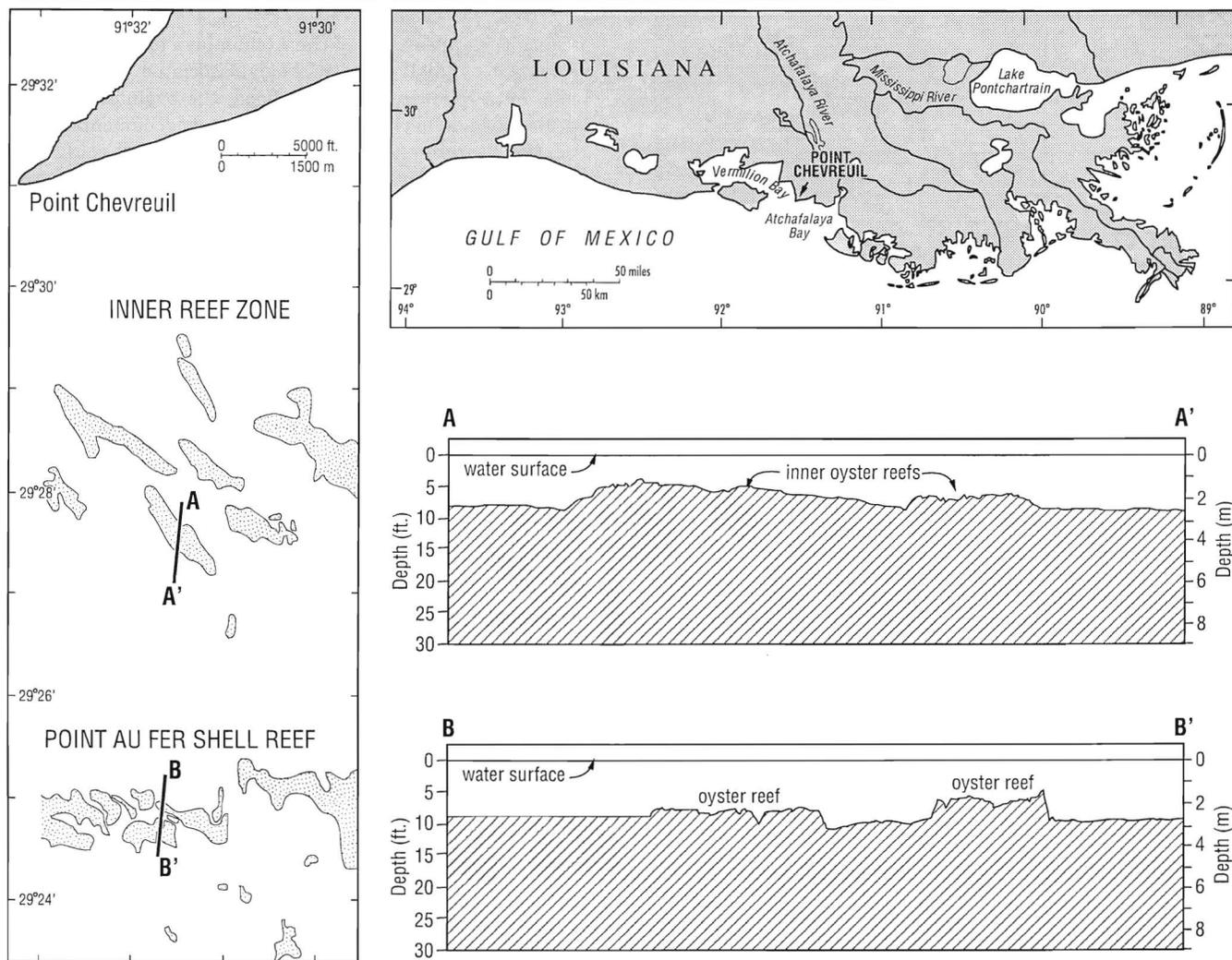
Figure 4. A plan-view map of western Atchafalaya Bay area showing the positive relief on both the inner oyster reef trend as well as the Point Au Fer shell reefs as represented on echo sounder profiles across these features (Thompson, 1951).
