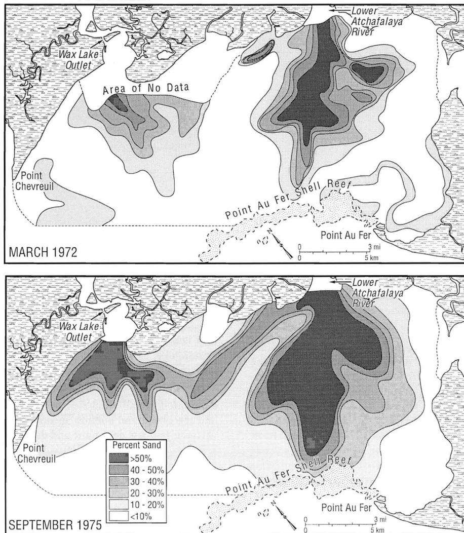
Figure 7. Distribution of sand concentration for Atchafalaya Bay bottom sediments as determined from USACOE (New Orleans District) samples (477 samples in 1972 and 160 samples in 1975), (Adapted from Roberts *et al.*, 1980).
