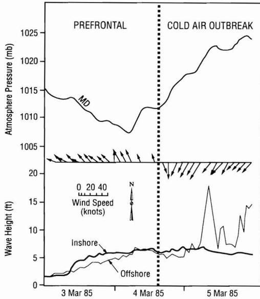
Figure 15. Surface measurements of barometric pressure, wind speed and direction and wave height made at 50 km (inshore) and 111 km (offshore) seaward of the eastern chenier plain during the passage of a cold front in March 1987 (modified from Roberts *et al.*, 1987). Note the onshore winds blowing from a southeasterly direction and low barometric pressure in the prefrontal phase while high pressure and strong northerly winds occur directly after the front passes.
