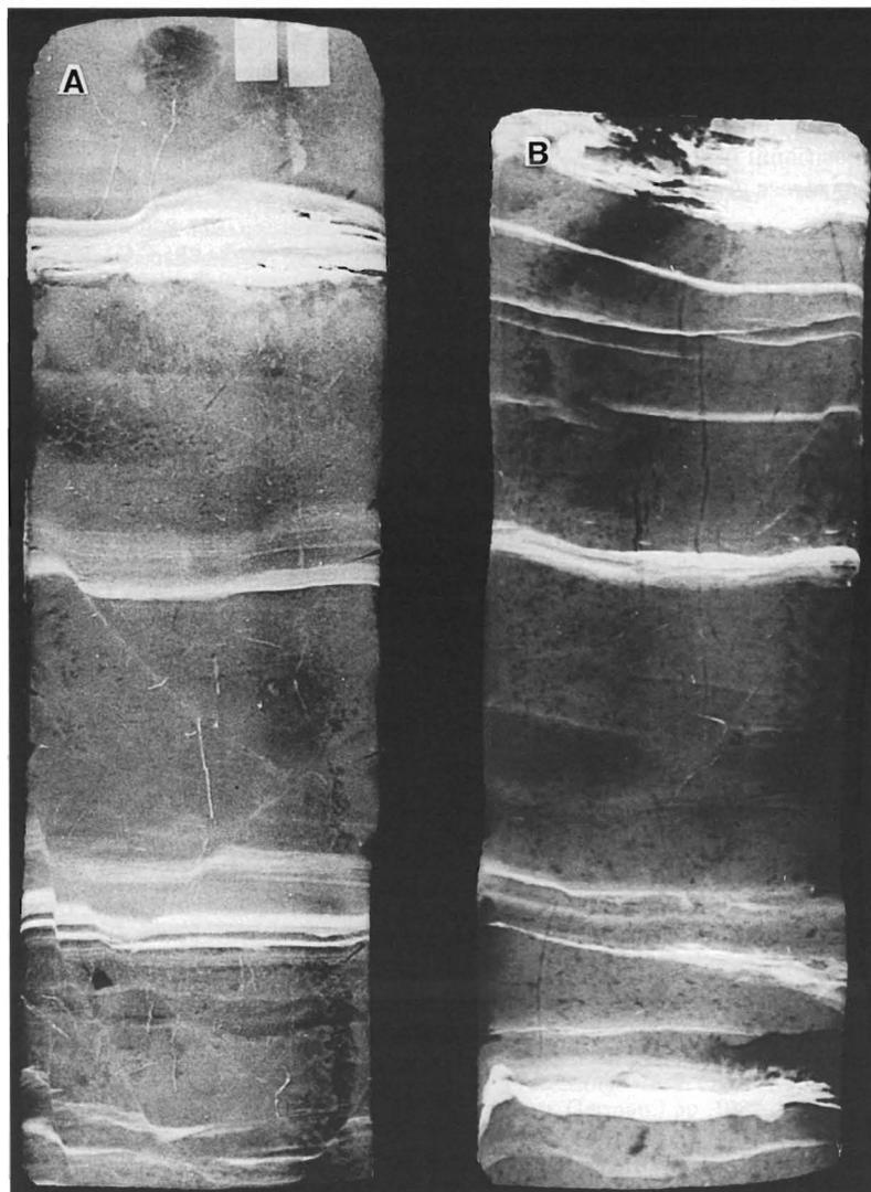
Figure 19. X-ray radiograph of a stacked series of cohesive and non-cohesive sediment couplets interpreted as having been deposited as a product of boundary layer sorting (Stow and Bowen, 1980) associated with sediment transport events during cold front passages. The core from which these subsamples were taken was acquired from the newly accreted mudflat illustrated in Figure 18b.
