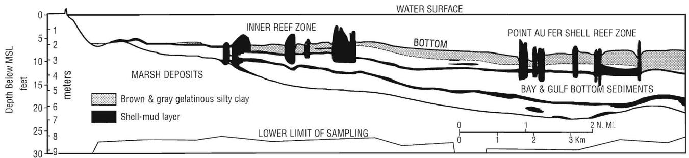
Figure 3. Cross section of Atchafalaya Bay from Pt. Chevreuil to the inner continental shelf south of the Point Au Fer shell reefs (see Figure 1 for general location). Note the abundance of oyster reefs along this transect and the seaward thickening wedge of "gelatinous mud" that equates to the first significant sedimentary deposits measured in Atchafalaya Bay and on the adjacent inner shelf associated with the Atchafalaya diversion (modified from Thompson, 1951).
