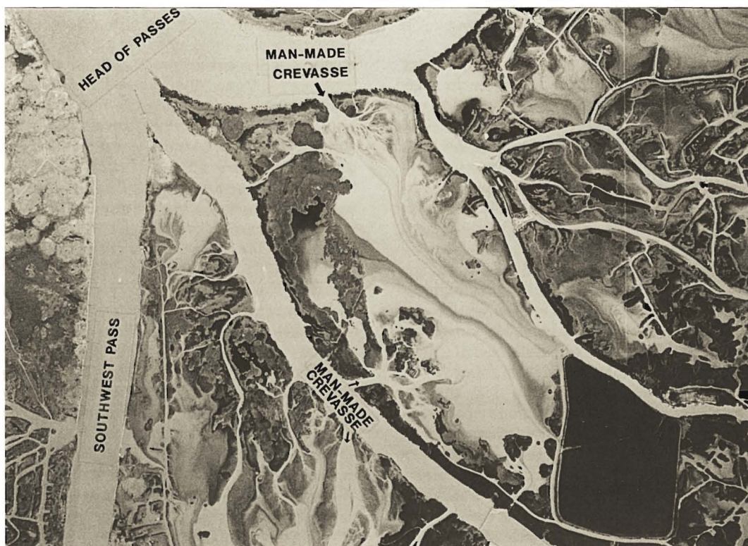
Figure 10. High altitude photograph of part of the Balize delta showing the positions of man-made crevasses along the South Pass and Pass-a-Loutre distributaries, taken in 1991.
