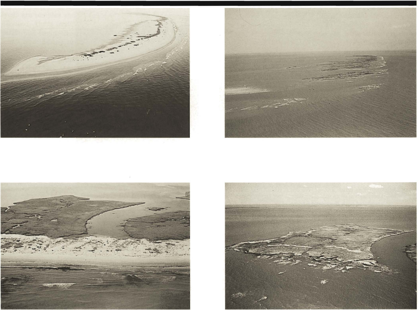
Figure 14. Barrier island response to storm generated waves caused by Hurricane Andrew (1992) along the Isles Dernieres, Louisiana. Note morphological condition of the barrier pre-Andrew (top left) and complete removal of coarser-grained material that exposes the mud core (top right) during and after landfall. Similarly, sand masses comprising the barriers and fronting the back barrier marshes (bottom left) were completely removed, leaving marshes prone to wave erosion (bottom right).
